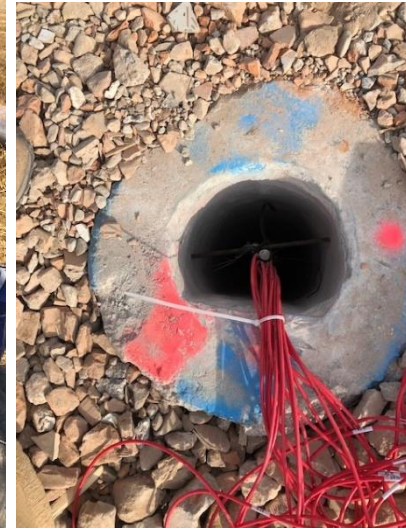
7 Strain gauged Piles
