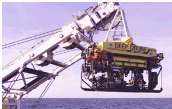
Deep Drone ROV Depth - 8,000 ft
