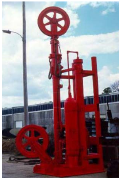
FADOSS 60-Kip Ship Motion Compensator
