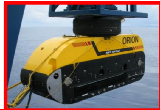
Orion21 Side Scan System Depth - 20,000 ft
