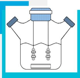
Smooth waves provide the effect of baffles at reduced shear stress.
